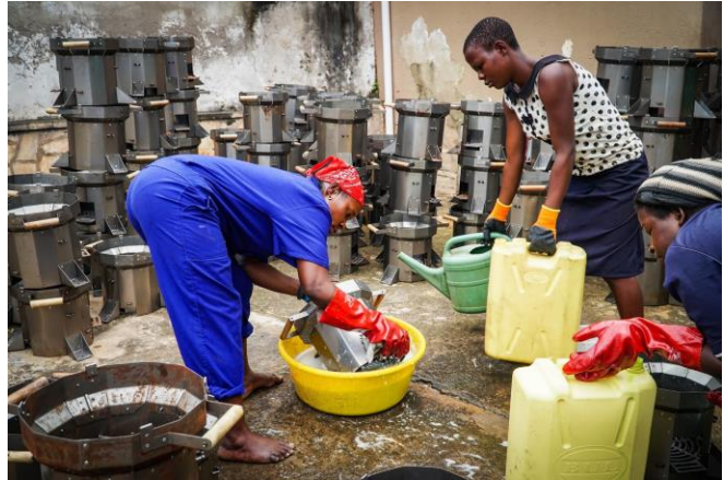
All the residue from the assembly process must be washed off before being painted
