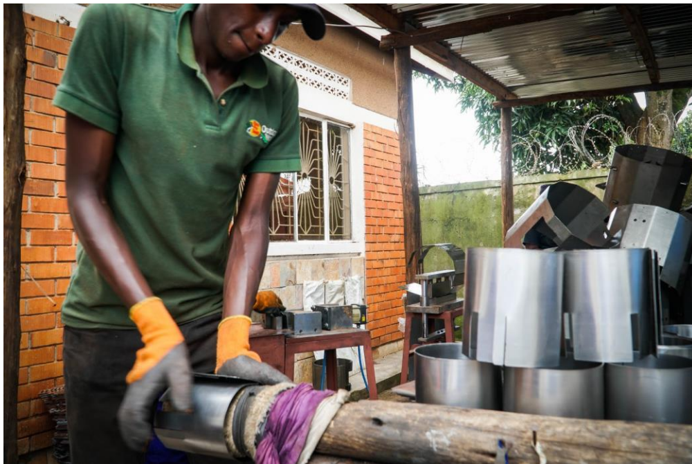
Abraham bends the fireboxes into a circular chamber
